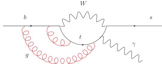
$$\left(\frac{\alpha_s}{\pi}\right)^n \log^n \frac{m_b^2}{M^2} \quad M = m_t, m_W : \text{leading logs (LL)}$$
